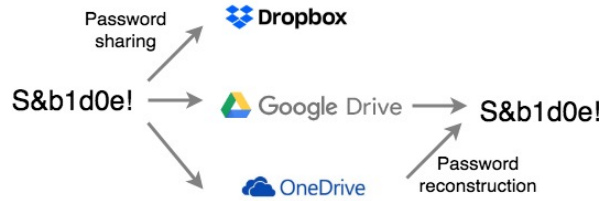
Figure 1: A password is divided in three shares, where each share is stored in a cloud; Reconstruction is possible from any two out of three shares
